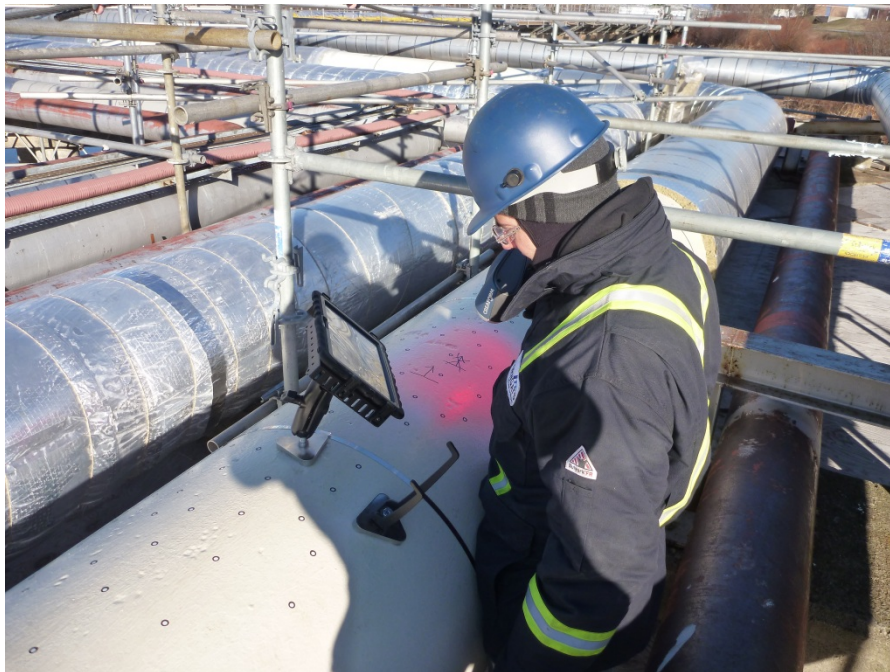
Figure 2: On-site inspection with the 3D laser scanner solution
