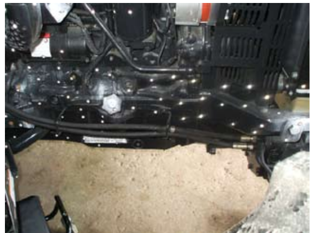
Scanned section of the tractor, for loader fitting
