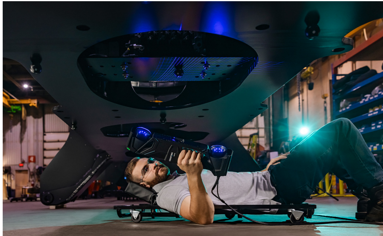
3D laser scanners with integrated photogrammetry are well suited for large parts and assemblies typically used in the heavy industry, aviation and shipbuilding.
