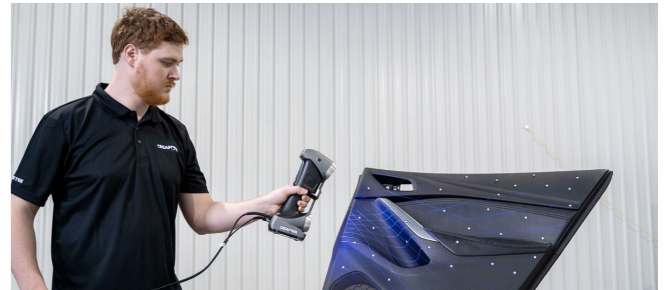
With a portable 3D scanner, parts can be measured right on the production floor. Image credit: Creaform.
