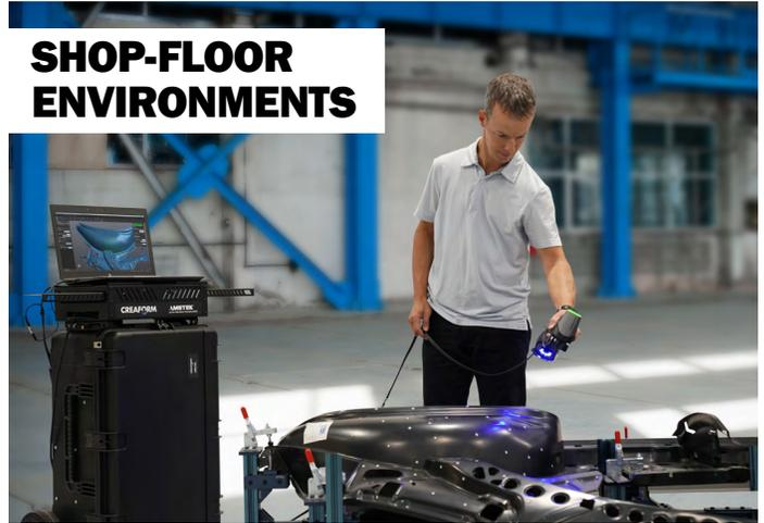
Creaform's portable workstation allows quality control teams of all skill levels to inspect parts at any stage of the production process—right on the shop floor. Greatly facilitating the setup of a portable 3D scanner anywhere in a manufacturing environment, this workstation is a powerhouse to help you improve your quality control efficiency and performance.
