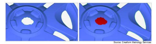
Figure 26: Damaged part/Complete fill hole.
