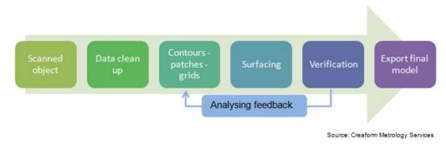
Figure 22: Representation of free form reverse engineering workflow.
