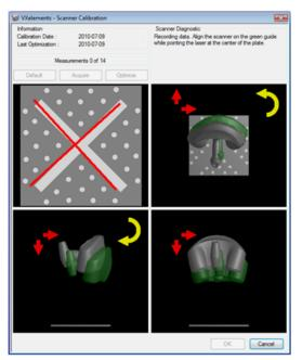
Source: Creaform Metrology Services Figure 36: Representation of the calibration procedure.
