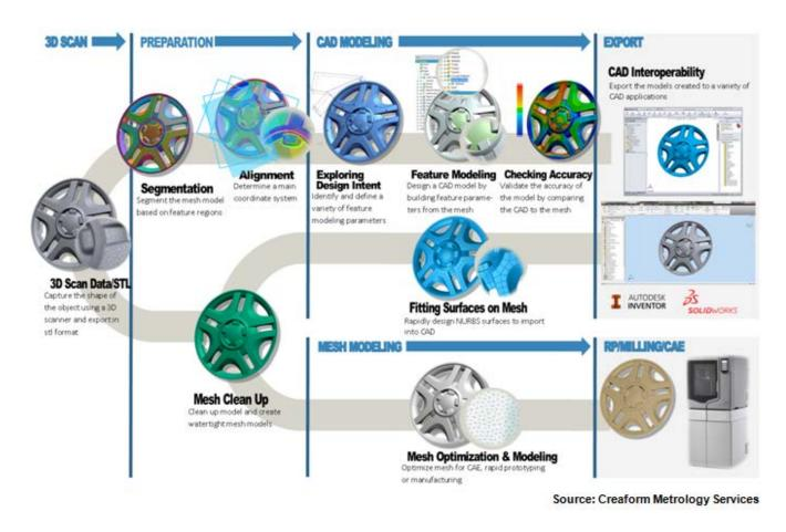
Figure 35: Representation of typical reverse engineering workflow.
