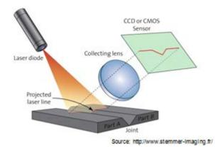
Figure 4: Principle of laser triangulation sensor.
