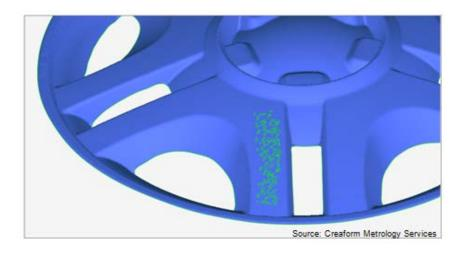
Figure 24: Representation of measurement noise (green triangles).
