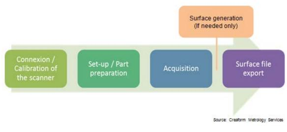
Figure 15: Representation of scanning workflow.
