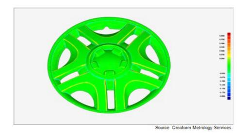
Figure 34: Representation of color mapping process for accuracy validation.
