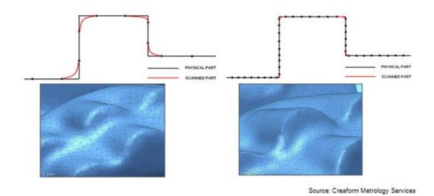
Figure 11: Difference between *Resolution* and *Accuracy*.
