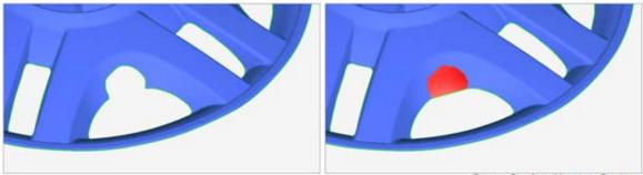
Figure 27: Damaged part/Partial fill hole.
