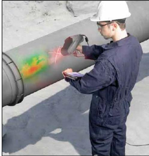
**Figure 1: EXAscan in the field with wireless tablet to visualise data**
