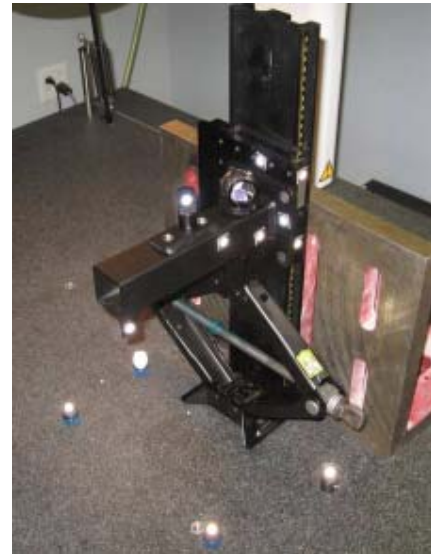
Figure 7: Experimental setup simulating slow movement on a vertical axis
