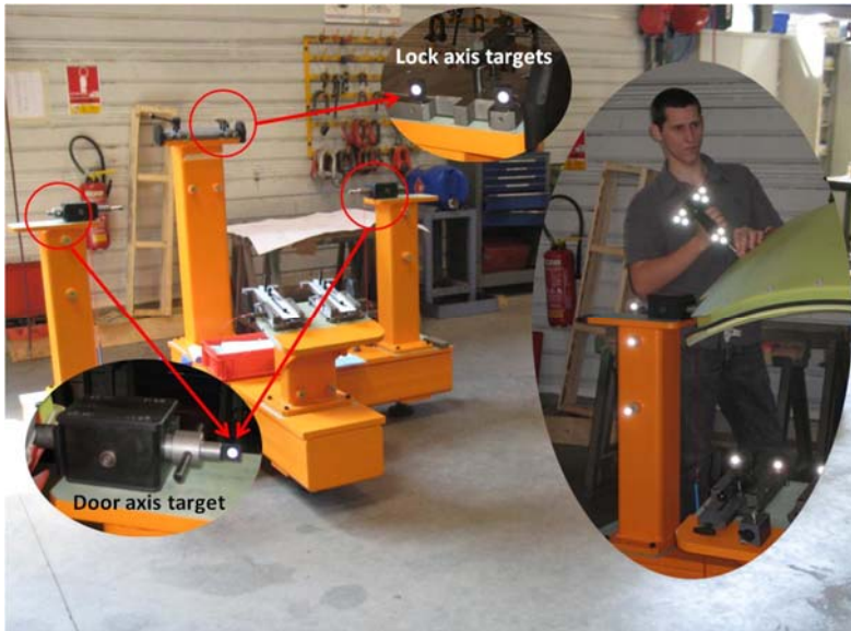
Figure 10: Example of a template designed to automate alignment and improve reliability in aeronautical parts measurement
