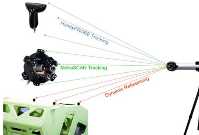
Figure 3: Operating principle of dynamic referencing
